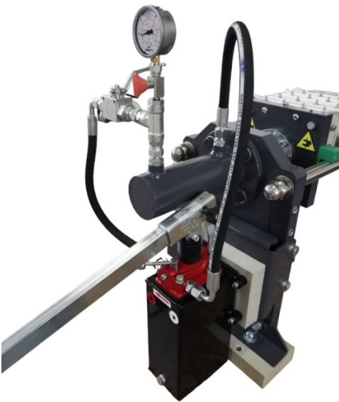
Picture n°5 - Hydraulic cylinder with manual pump, lever and oil tank
